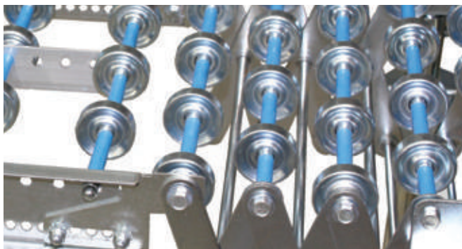
Roller conveyor width 300 mm
