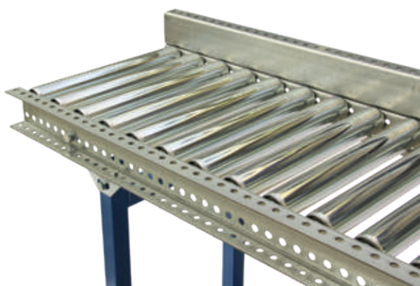
Side guides, galvanised U-profile, 40 / 80 / 40 x 3 mm, guide height up to 75 mm above roller, double-sided
