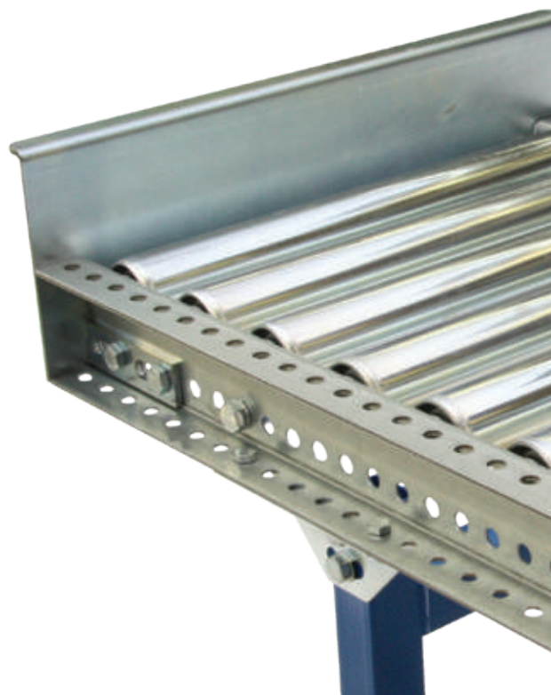
Side guides, galvanised U-profile, 40 / 80 / 40 x 3 mm, guide height up to 75 mm above roller, single-sided
